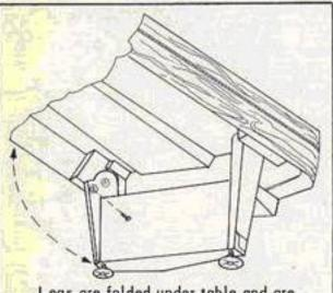
Legs are folded under table and are swung into position and bolted there for rapid set up and unsurpassed support. Legs never leave table.
