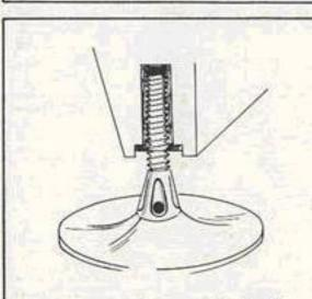
New Five inch die cast leg leveler with 1/2" thick threaded portion. Leveler screws into special die cast "T" nut 2-1/8" long.
