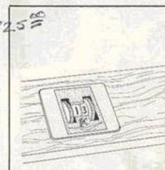
Two die cast chrome plated scoring markers recessed into Formica top frame.
