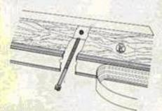
Cushion moldings are held to top frame by hex head slotted machine screws that screw into 'T' nuts imbedded in cushion molding. No more broken screws or stripped wood, (special spin tight provided with all tables, fits rail screws as well as all other hardware) Aluminum molding between cabinet and top frame hides all screws.
